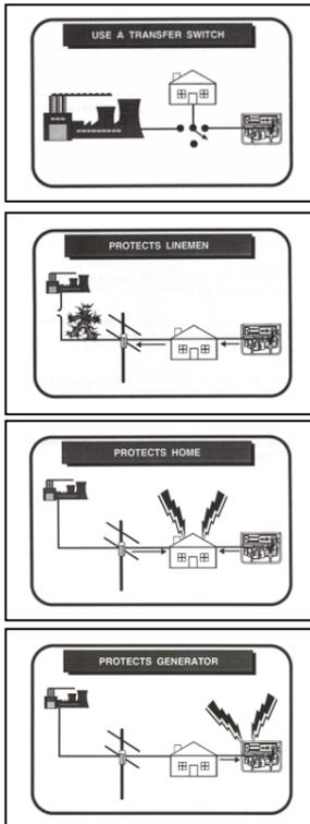
A transfer switch prevents both the utility power and generator power from being connected at the same time.
